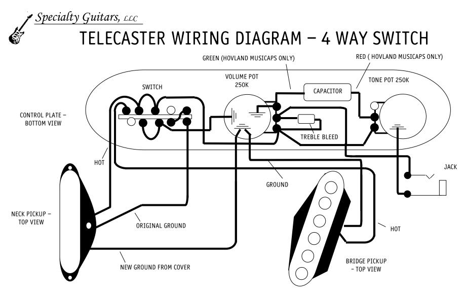
IF YOUR PICKUP HAS A COVER, YOU MUST LIFT THE EXISTING GROUND AND ADD AN ADDITIONAL GROUND WIRE.
